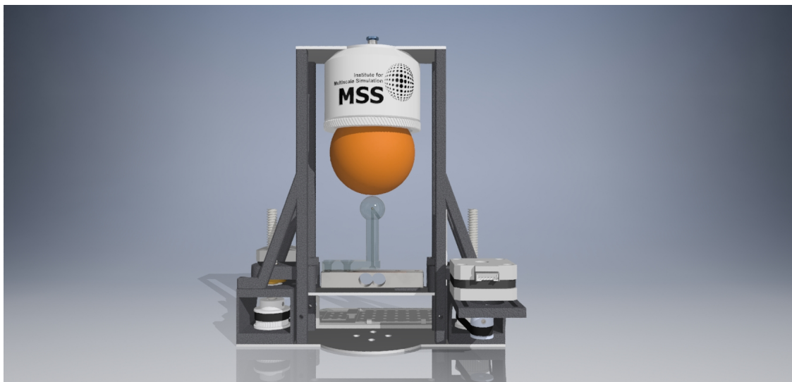
Figure: Experimental setup for automatic holding force measurements.
