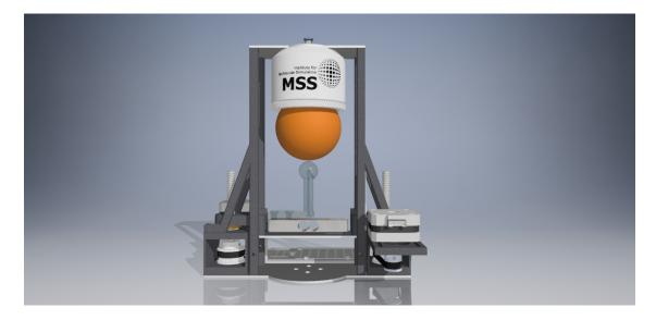
Figure: Experimental setup for automatic holding force measurements.
