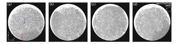
**Figure:** Snapshots of the packing of  $\varphi = 0.57$  and A = 7 mm at the middle of (a) cycle 1, (b) cycle 5, (c) cycle 9 and (d) cycle 13. In the inset of (d) the oscillation path of the amplitude A = 10 mm is drawn up to scale.
