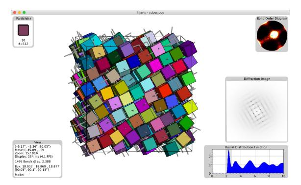
**Figure:** Screenshot of injavis showing a snapshot of a simulation of hard cubes. (top left) particle module; (top right) bonds module; (middle right) diffraction module; (bottom left) view module; (bottom right) RDF module
