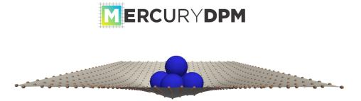
Figure: Snapshot of a simulated membrane with the spring system by MercuryDPM.
