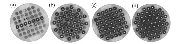
**Figure:** Rotational granular gas lattices. (a) two neighbors; (b) three neighbors; (c) four neighbors; (d) six neighbors. Also, the lattice constant, a, and the clearance,  $R = r_h - r_l$ , can be chosen
