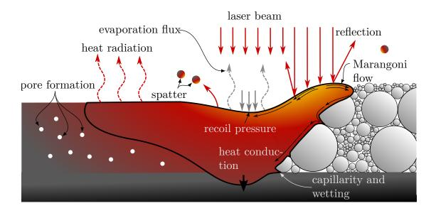
Figure: Physical phenomenon arising in laser-metal processing.
