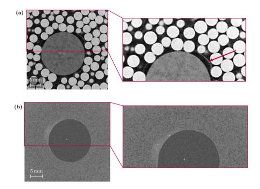
**Figure:** Tomogram slices for (a) (d = 4.0 mm) particles and (b) (d =  $120 \mu$ m) particles after evacuation of the gripper. The images on the right side are magnifications of the original tomogram slices. The arrow notes a region where the membrane is not in contact with the surface of the object.
