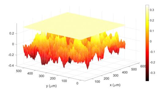
**Figure:** Contact between a smooth and a rough surface. The colour map shows the elevation in  $\mu$ m measuring from the average height of the rough surface.
