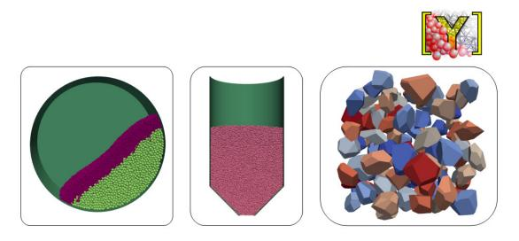
Figure: DEM applications in YADE; rotating drum, silo flow and sample of polyhedral particles.
