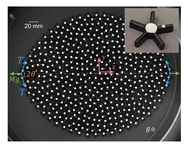
**Figure:** Photograph of the pressure-controlled experiment with star-shaped particles (inset). Airfluidized particles are enclosed by a boundary made of a chain of particles on a thin flexible thread. The left end is pulled with a controlled force while the right end is anchored.
