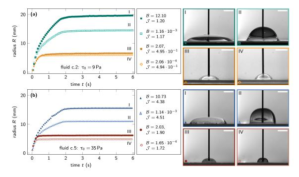
**Figure:** Radius R(t) of the droplets as a function of time, comparing the same fluids on-ground (labeled 1*g*, filled marks) and under microgravity conditions ( $\mu g$ , empty marks). Pictures are taken at the last instant before the end of the experiment. In all pictures, the scale bar represents 8 mm.
